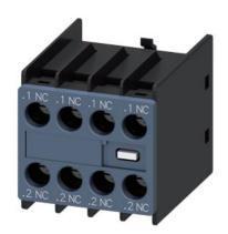
auxiliary switch, on the front, 4 NC, .1/.2, .1/.2, .1/.2, .1/.2, current path: 1 NC, 1 NC, 1 NC, 1 NC, screw terminal, for contactors 3RT2 and contactor relays 3RH2
