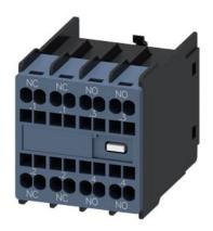
auxiliary switch, on the front, 2 NO + 2 NC, .1/.2, .1/.2, .3/.4, .3/.4, current path: 1 NC, 1 NC, 1 NO, 1 NO, spring-loaded terminal, for contactors 3RT2 and contactor relays 3RH2
