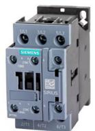
Contactor AC 110 V 50/60 HZ AC3 11 kW 400 V AUX contacts 1 NO +1 NC 3-pole, size S0 screw terminal
