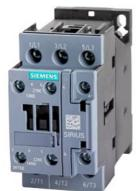
Contactor AC 220 V 50 HZ AC3 15 kW 400 V AUX contacts 1 NO +1 NC 3-pole, size S0 screw terminal
