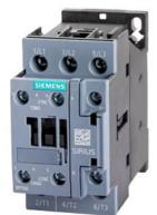
Contactor AC 220V 50/60 HZ AC3 18,5 kW 400 V AUX contacts 1 NO +1 NC 3-pole, size S0 screw terminal
