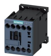
Contactor DC 24 V AC3 3 kW 400 V AUX contacts: 1 NC 3-pole, size S00 screw terminal
