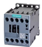
Contactor AC 24 V 50/60 HZ AC3 3 kW 400 V AUX contacts: 1 NO 3-pole, size S00 screw terminal
