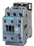
Contactor DC 24 V AC3 11 kW 400 V AUX contacts 1 NO +1 NC 3-pole, size S0 screw terminal
