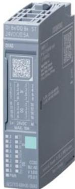
SIMATIC ET 200SP, digital combined module, DI 8x/DQ 8x24 V DC/0.5 A standard, DI: sink input, (sinking input), DQ: source output (sourcing output) suitable for BU type A0, color code CC00, substitute value output for DQ, module diagnostics for: short circuit to L+ and M, wire break, supply voltage
