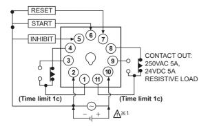
%1: AC/DC voltage: 100-240VAC 50/60Hz, 24-240VDC
