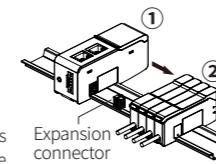
03. Push the side connector on the right side of the converter toward the expansion connector of the amplifier to make the connection. Check that the connectors are securely and tightly connected.
