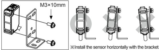
※Install the sensor horizontally with the bracket.
