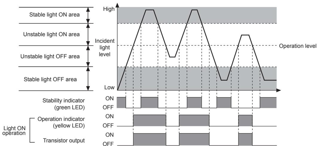
※The waveforms of 'Operation indicator' and 'Transistor output' are for Light ON operation. The waveforms are reversed for Dark ON operation.
