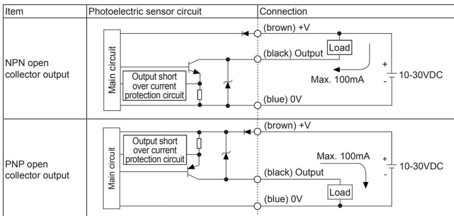
※If short-circuit the control output terminal or supply current over the rated specification, normal control signal is not output due to the output short over current protection circuit.
