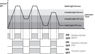
· In Dark ON mode, the waveforms are reversed
