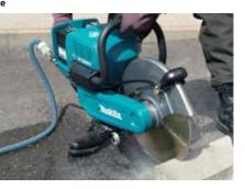
Abrasive cut-off wheel for Metal 355 x 4.3 x 25.4 A24T
