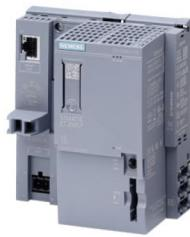
SIMATIC DP, CPU 1510SP F-1 PN for ET 200SP, central processing unit with 300 KB work memory for program and 1 MB for data, 1st interface: PROFINET IRT with 3-port switch, 6 ns bit performance, SIMATIC Memory Card required, BusAdapter required for port 1 and 2
