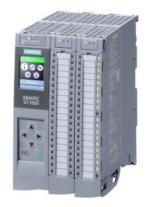
SIMATIC S7-1500 Compact CPU CPU 1511C-1PN, central processing unit with working memory 175 KB for program and 1 MB for data, 16 digital inputs, 16 digital outputs, 5 analog inputs, 2 analog outputs, 6 high speed counters, 4 high speed outputs for PTO/PWM/frequency output 1. interface: PROFINET IRT with 2 port switch, 60 NS bit-performance, incl. front connector push-in, SIMATIC memory card necessary
