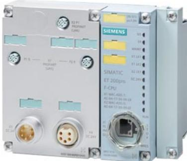
SIMATIC DP, CPU 1513pro F-2 PN for ET 200pro, central processing unit with 450 KB work memory for program and 1.5 MB for data, 1st interface: PROFINET IRT with 3-port switch, 2nd interface: PROFINET RT, 40 ns bit performance, Degree of protection: IP65/67, SIMATIC Memory Card required connection module required
