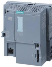
SIMATIC DP, CPU 1514SP T-2 PN for ET 200SP, central processing unit with 900 KB work memory for program and 3.5 MB for data, 1st interface: PROFINET IRT with 2-port switch, 2nd interface: PROFINET RT 6 ns bit performance, SIMATIC Memory Card required, BusAdapter required for 1 interface
