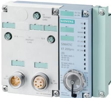
SIMATIC DP, CPU 1516PRO-2 PN for ET 200pro, Central processing unit with Work memory 1 MB for program and 5 MB for data, 1st interface: PROFINET IRT with 3-port switch, 2nd interface: PROFINET RT, 10 ns bit performance, degree of protection: IP65/67, SIMATIC Memory Card required, Connection module required
