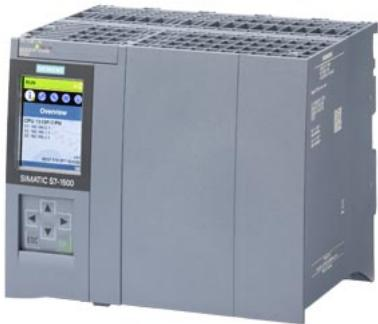
SIMATIC S7-1500, CPU 1518F-3 PN, central processing unit with 18 MB work memory for program and 150 MB for data, 1st interface: PROFINET IRT with 2-port switch, 2nd interface: PROFINET IRT with 2-port switch, 3rd interface: Ethernet, 0.3 ns bit performance, SIMATIC Memory Card required
