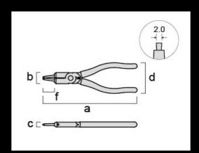
The tip of the claw is processed into a reverse taper shape, so it catches the snap ring securely and does not slip off.
