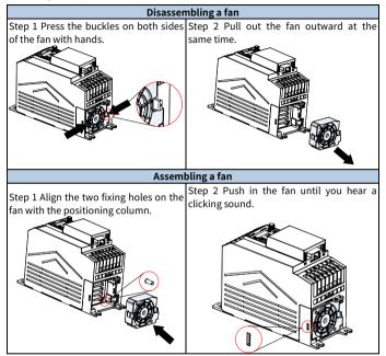
Note: Before disassembling or installing the VFD, stop the VFD, cut off the power, and wait at least 5 minutes.
