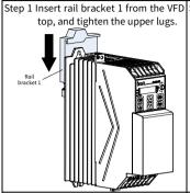
Step 1 Insert rail bracket 1 from the VFD Step 2 Insert rail bracket 2 from the VFD bottom, and tighten the lower lugs. Rail bracket 2
