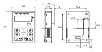
Figure D-5 Keypad openings without a bracket
