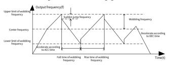
Wobbling frequency = Central frequency (Set frequency) x P08.15 (Amplitude of wobbling frequency)
