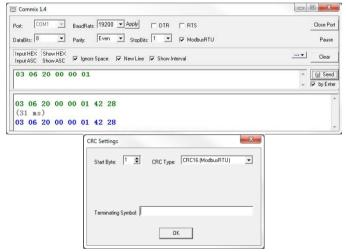
Set Port to COM1. Set BaudRate consistently with P14.01. DataBits, Parity, and StopBits must be set consistently with P14.02. If the RTU mode is selected, choose Input HEX and Show HEX. To implement automatic CRC, you need to choose ModbusRTU, and set Start Byte to 1 and CRC Type to CRC16 (MODBU SRTU) in the CRC Settings window. After the automatic CRC is enabled, do not enter CRC in commands. Otherwise, command errors may occur due to repeated CRC.
