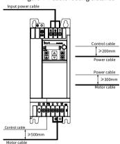
Figure 4-4 Cable routing distance
