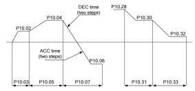
Note: The sign of multi-step speed determines the running direction of simple PLC, and a negative value means reverse running. ACC time means the time needed if the VFD speeds up from 0Hz to the max. output frequency (P00.03). DEC time means the time needed if the VFD speeds down from the max. output frequency (P00.03) to 0Hz. Select corresponding ACC/DEC time, and then convert 16-bit binary number into hexadecimal number, finally, and then set corresponding function codes.
