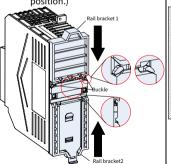
Step 3 Fasten rail brackets 1 and 2. Step 4 Place the VFD with brackets vertically on the DIN rail, and push sheet metal lock catch upwards to make it tightly engage with the rail.
