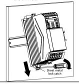
the DIN rail bracket inward, and then pull out rail brackets 1 and 2.
