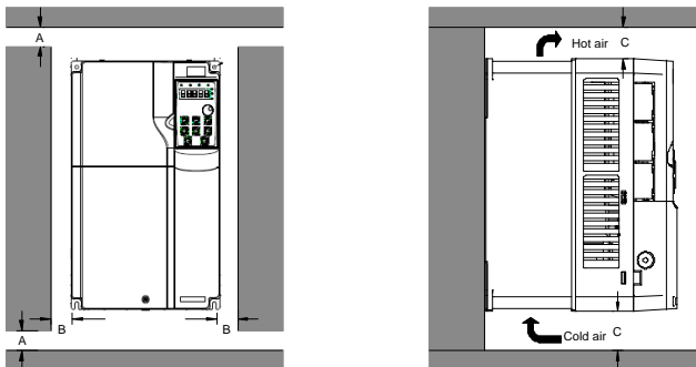
Figure 4-3 Installing one VFD
