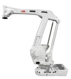
Thanks to its state-of-the-art 4-axes design, customers can look forward to a speedy machine that combines a 3.15 meter reach with a 250 kg payload, making it ideal for palletizing bags, boxes, crates, bottles and more. In fact, ABB is set to reinforce its position as the sole global supplier of complete robotbased packaging line automation.
