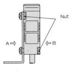
OScrew tightening torque should be 8kgf · cm(0.8 Nm)max.
