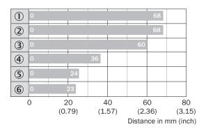
$\begin{tabular}{ll} \hline & Max. sensing range $S_n$, flush or non-flush installation, \\ & non-magnetizable material \\ \hline \end{tabular}$
