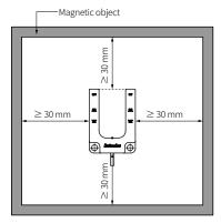
• Install the switch to the position where the center of the switch and the target be exactly horizontal and vertical.
