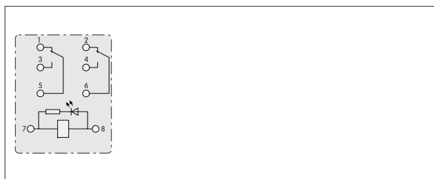
Connection diagram (bottom view) 2Z(D)
