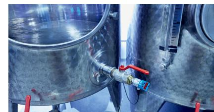
High precision from pressures of 0.4 bar means the device is particularly economical for hydrostatic level measurements with low water columns.
