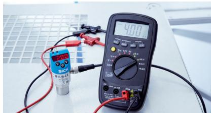
The scalable analog output allows for individual adaptation to the pressure range relevant for the application.
