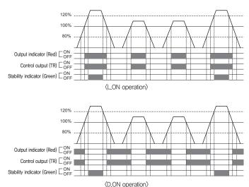
Stability indicator becomes ON when an amount of light exceed the operation level and becomes 120% (stable L\_ON area). It can be used as the environmental change after setup or level down during operation and initial operation check.
