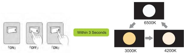
To cycle through between different color temperature, toggle light switch from on-off-on within 3 seconds.
