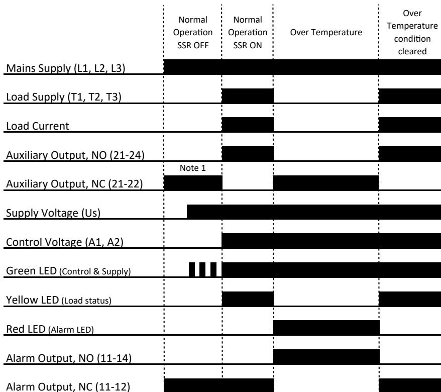
Note 1: For the AC external supply versions (RGC..A..A), the Auxiliary output, NC (21-22) will be closed only when the external supply Us is present.
