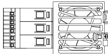
Housing width tolerance +0.5mm, -0mm as per DIN 43880.
