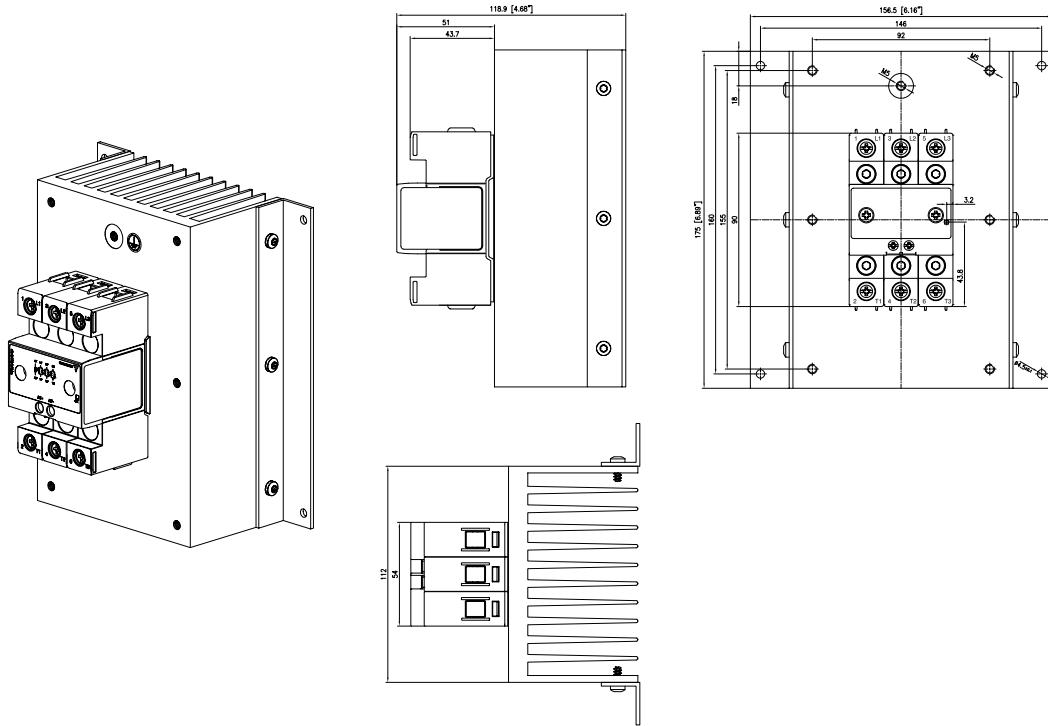
Housing width tolerance +0.5mm, -0mm as per DIN 43880.
