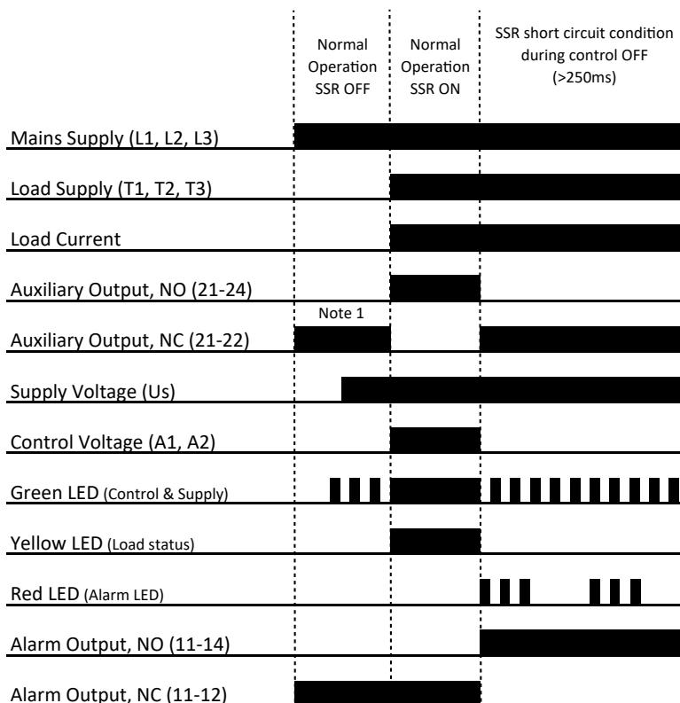
Note 1: For the AC external supply versions (RGC..A..A), the Auxiliary output, NC (21-22) will be closed only when the external supply Us is present.
