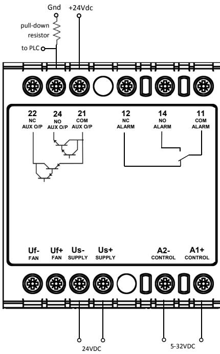
Connection of normally open auxiliary output (24-21) in a 'pnp' style
