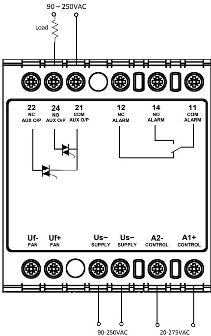
Connection of normally open auxiliary output (24-21) to an AC load
