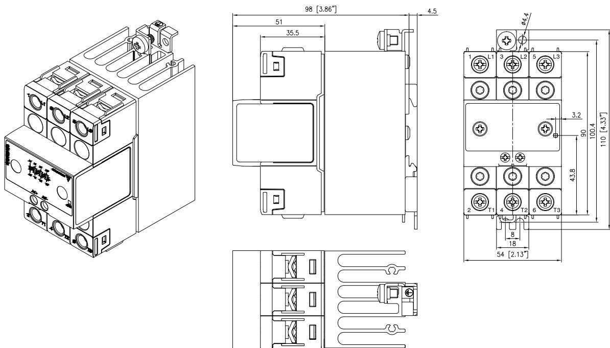
Housing width tolerance +0.5mm, -0mm as per DIN 43880.
