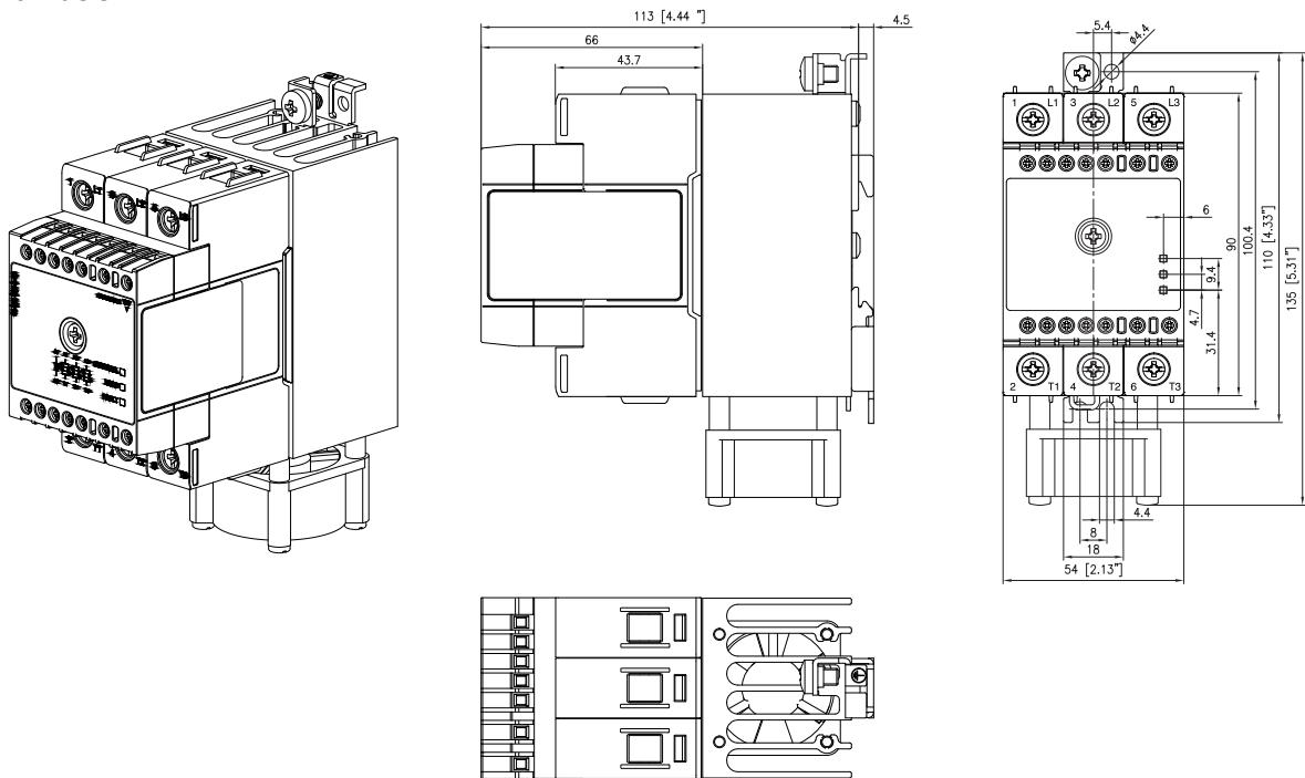
Housing width tolerance +0.5mm, -0mm as per DIN 43880.
