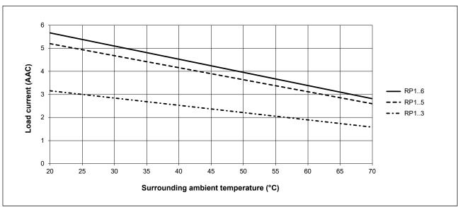
When used at full load current, the relays must be placed vertically. If more than one relay is mounted, please allow a minimum distance of 20 mm in between for sufficient air cooling.
