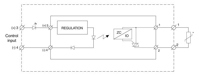
\* The varistor is not included in the solid state relay. Connecting a varistor across terminals 1-2 helps protect the solid state relay against damages by over-voltage.
