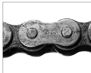
Fig. 35 Hydrogen embrittlement cracking
