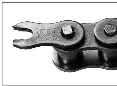
① Static fracture Applying load to a link plate beyond its breaking load will cause it to stretch and then break.
