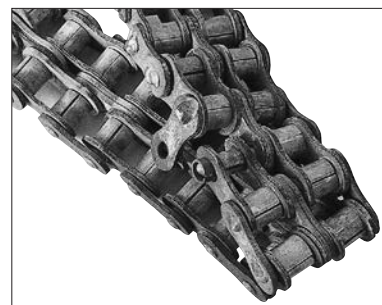
Fig. 34 Corrosion of stainless steel roller chain
