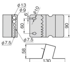
The material is 18-8 stainless steel which has excellent corrosion resistance, which is also used for food equipment.
