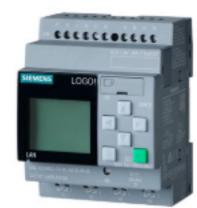
\*\*\* spare part \*\*\* LOGO! 24RCE, logic module, display PS/I/O: 24V AC/DC 24V/relay, 8 DI/4 DO, memory 400 blocks, modularly expandable, Ethernet, integr. web server, data log, user-defined web pages, standard microSD card for LOGO! Soft Comfort V8 or higher, older projects executable
