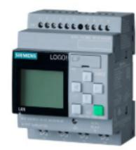
\*\*\* spare part \*\*\* LOGO! 230RCE,logic module, display PS/I/O: 115V/230V/relay, 8 DI/4 DO, memory 400 blocks, modularly expandable, Ethernet, integr. web server, data log, user-defined web pages, standard microSD card for LOGO! Soft Comfort V8 or higher, older projects executable
