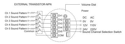
• Wiring terminal on the back side of the product.
