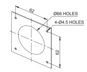
• First, machine taps or holes on the mounting surface(1).
