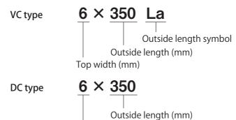
The VC type has a size indication on the back face of the belt; however, the DC type does not have the indication.
